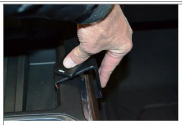
2. Press down on the right side of the ProClip and, at the same time, press to the left on the bottom edge of the ProClip to hook the lower edge of the ProClip under the right side panel of the center console.
